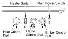
Figure 3 - Electric Stove Control Panel
